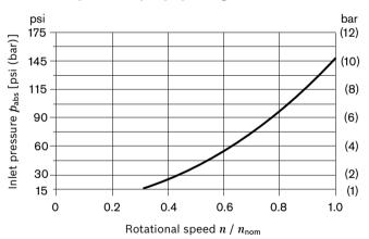
This diagram is only valid for the optimum viscosity range of  $v_{opt}$  = 170 to 73 SUS (36 to 16 mm<sup>2</sup>/s).
