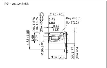
$_{\mbox{\scriptsize 1)}}\,$  ANSI B92.1a, 30° pressure angle, flat root, side fit, tolerance class 5
